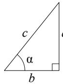
$$\begin{aligned}\sin \alpha &= \frac{a}{c} \\ \cos \alpha &= \frac{b}{c} \\ \operatorname{tg} \alpha &= \frac{a}{b}\end{aligned}$$
